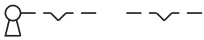
18 Keylock switch actuator 3 positions page 16 | Keylock switch actuator 3 positions, flush mounting page 22
