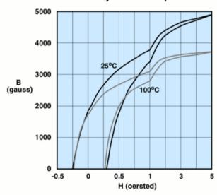
Measured on an 18/10/6mm toroid at 10kHz.
