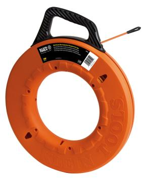
Klein Tools' Multi-Groove Fiberglass Fish Tapes feature a low-friction, easy feed design. The grooved profile and fiberglass core provide rigidity for long distances and less surface contact with wires when pushing through crowded conduit. The non-conductive fish tape and non-conductive eyelet tip offer added protection against shock from energized sources.
