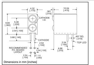
Standard Polarity shown in drawing: Cathode right
