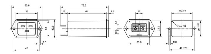
Rear side mounting with pre-formed, threaded holes for M3 screws
