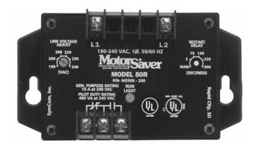
**Model 50R** Single Phase Voltage Monitor has a voltage sensing circuit which constantly monitors the single phase power for a low voltage condition. Single phase motors on fans, compressors, air conditioners, heat pumps, well pumps, sump pumps, and small conveyor motors are all applicable to the Model 50R.
