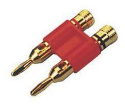
Banana Plug Pair Commonly used for test equipment and speaker connections. This paired banana plug set provides secure, trouble free connections with all standard spaced banana jacks and binding posts. Popular for use on speaker terminal plates, amplifier outputs, volt meters, power supplies, function generators and counters, anything that has standard 0.75" center spacing.
