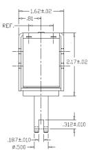
Solenoid shown energized with plunger fully seated
