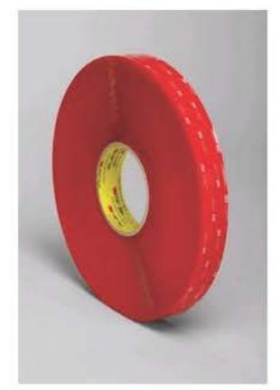
3M™ VHB™ Tape 4910 is a clear double-sided, pressuresensitive, acrylic tape with PE film liner. 40 mil thick.
