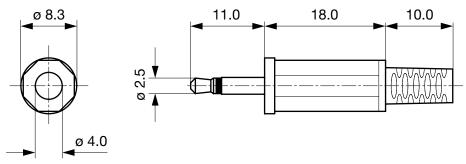
Cable diameter max. 4.0 mm
