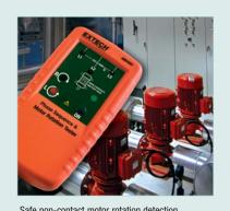
Safe non-contact motor rotation detection
