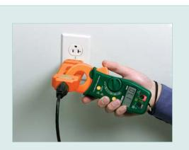
Provides easy and safe measurement of current without the need to cut off the plug and separate the conductors
