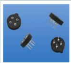
Fully molded compact construction. Speeds transistor assembly. Incorporates ultra high quality, closed entry, sleeve type contacts. Accepts .016 (.41) to .020 (.51) diameter leads or .010 (.25) × .018 (.46) rectangular transistor leads.
