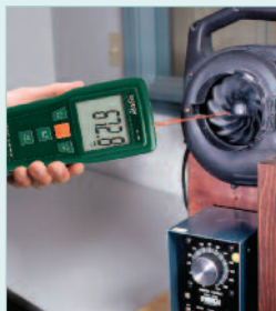
Photo Tachometer function measures the speed of rotating objects without contacting the surface by using a laser beam and reflective tape
