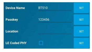
**Device Name –** Used to assign a user-friendly name to the sensor
