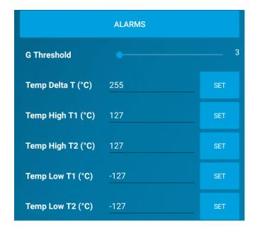
**G Threshold** – Sets the acceleration threshold on the sensor. The lower the number, the lower amount acceleration acted on the device is required to trigger the alarm.
