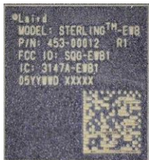
Figure 1 Sterling-EWB Base SiP module (453-00012)
