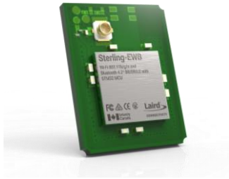
Figure 2: Sterling-EWB U.FL module (453-00013)
