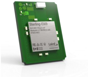
Figure 3 Sterling-EWB chip antenna module (453-00014)
