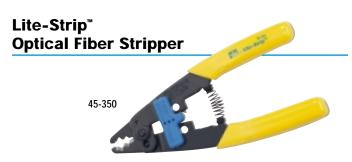
V-notch blades strip a wide range of outer cable jacket. Precisionground, replaceable knife-type blades strip tight buffer tube insulations (900µm). Also strips mechanically strippable coatings from 250 microns to 900 microns.
