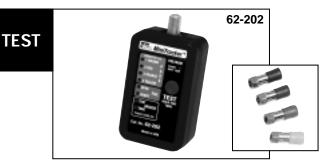
Testing of coaxial cable generally consists of checking for opens or shorts in the cable. Use the **IDEAL MiniTracker Tester** (62-202) to test for opens or shorts in the cables terminated with F-connectors. This tester can be used through a standard splitter or individual runs of cable and also to trace cable for identifying cable runs.
