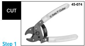
Cutting of coaxial cable requires the use of a shearing type or rounded blade cable cutter, like the IDEAL Data T®-Cutter (45-074). Cut the coaxial cable to the proper length needed for your application. Note: Diagonals or side-cutters will deform the cable and may affect the performance. However, if your coaxial cable has a center conductor made of steel, it is recommended you use a diagonal cutter.
