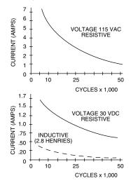
Voltage and Load: As listed in the chart One cycle is 360° rotation and a return through all switch positions to the starting position. The data for the curves was measured at sea level, 25°C and 68% relative humidity.
