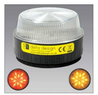
CE – certified to EMC directive 2004/108/EC. Complies with low voltage directive 2006/95/EC. High voltage transient and polarity reversal protected. Operating temperature:  $-20^{\circ}$ C to  $+55^{\circ}$ C.
