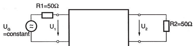
Fig. 4. Four pole network with real termination
