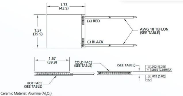
Solder Construction: 271°C, Proprietary
