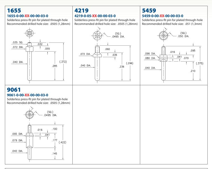
Recommended drilled hole sizes are prior to plating of the PCB and based on typical copper deposition of .5 - 1 oz. This results in a reduction of hole size by approximately .0015" - .003". Depending on surface plating, typical finished hole sizes are .003" - .005" smaller than drilled hole sizes. The finished hole size tolerance for press-fit applications should be specified as +/- .002"
