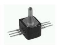
**Pressure Sensors: Measurement** Type: Gage; Signal Conditioning: Amplified; Pressure Range: 0 psi to 500 psi; Port Style: Straight O-ring interface
