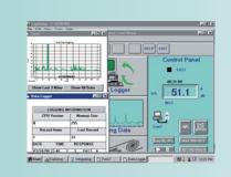
Leq and SEL measurements with built-in datalogger and PC interface. Datalogs up to 32,000 readings using included software and USB cable.
