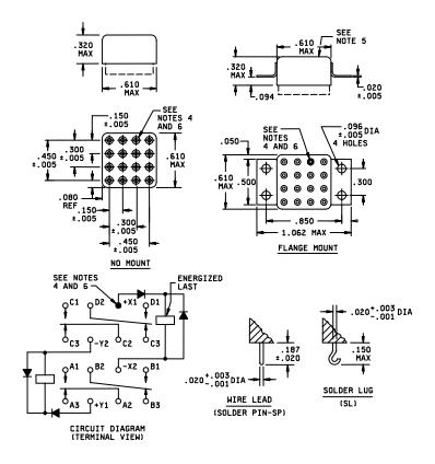
FIGURE 1. Configuration and circuit diagram.
