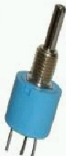
392 Series Industrial Potentiometer, Conductive Plastic Element, PC Terminals, 0.5 W Power Rating, 500 kOhm Resistance Value
