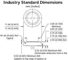
(applies to top edge of gasket or edge of crimp, whichever is higher)
