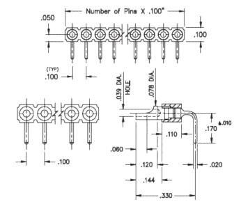
**Description:** Interconnect Header Solder Tail Pin Header SolderCup Head Single Row Through Hole Plating Code: 10 Shell Plating: 10  $\mu$ " Gold over 100  $\mu$ " Nickel
