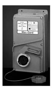
MaxGard® NEMA 4x interlocks are ideal for demanding non-hazardous areas where dust, dirt, moisture and corrosion might be a problem-such as shipyards, food processing facilities, manufacturing operations or similar areas.
