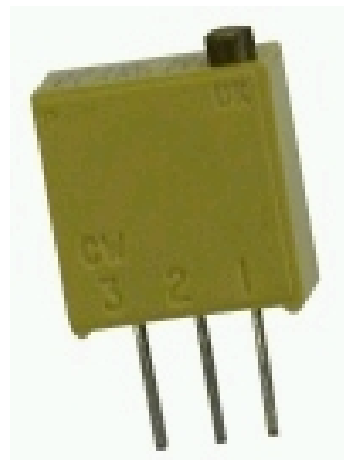
364 Series Trimmer, 5 kOhm, 0.5 W, 25 Turns, Square Body, Vertical Shaft
