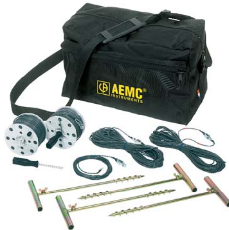
Ground Test Kit for 4-Point testing includes carrying bag, two 300 ft color-coded leads on spools, two 100 ft color-coded leads, four 16" auxiliary ground electrodes, one 16 ft lead with Mueller® clip and one 100 ft tape measure Catalog No. 2130.63
