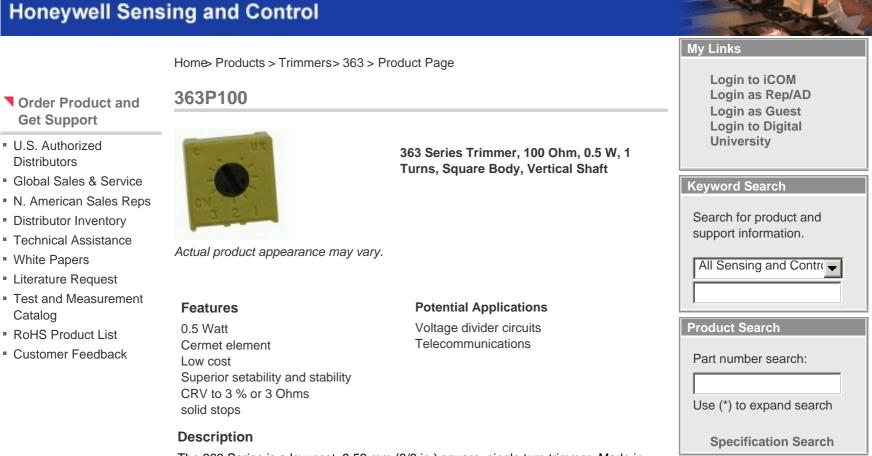
The 363 Series is a low cost, 9.53 mm (3/8 in.) square, single turn trimmer. Made in accordance to MIL-R-22097 standards, the 363 is sealed for cleaning in common solvents.
