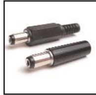
30-374 Bakelite Barrel 30-374-P With Strain Relief. Coax power plug. 2.5 mm I.D. 5.5 mm O.D. 9.5 mm long. .15" cable opening.
