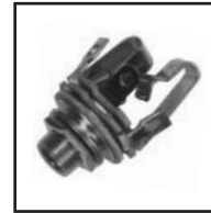
30-400 Stereo 30-411 Mono 3 Circuit 1/4" Open, Mono or Stereo Audio Jack. .35" x .29" bushing. .36" hole size, will work with standard .375" hole.
