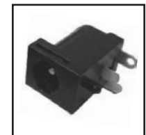
30-616-2.1 30-616-2.5 Locking DC power coax jack with N/C switch on sleeve side of the connector. Insert 30-617 plug and twist clockwise to lock.
