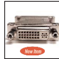
35-710 DVI-I to DVI-I Female to Female Coupler. Shielded di-cast case handles 5 pin analog and 24 pin digital signals. gold plated contact pins. Used for inline or chassis mount. Fits in standard DB15 d- sub cutout. Overall length .93" For wall mounting use Calrad p/n 30-598.
