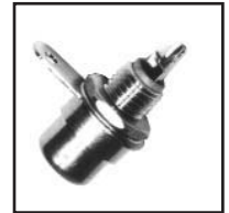
30-428-COLOR Nickel 30-428G-COLOR Gold Nickel plated RCA Audio Jack with hex nut and solder lug. Single hole mount. 1/4" hole. Bushing length .25" Available with black, blue, green, red, white and yellow inserts.
