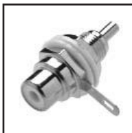
30-300-COLOR RCA chassis mount Audio Jack. Gold plated with teflon insulator mount. Fits 5/16" hole. Bushing length .43" Available with black, red, white and yellow inserts. Please specify color when ordering.
