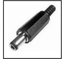
30-375 DC coax power plug. 3mm I.D., 6.3mm O.D., 9.5mm long. With strain relief. .20" cable opening.
