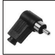
30-384 Right angle RCA Audio Plug. Solderless connector with cable clamp. .19" cable opening.
