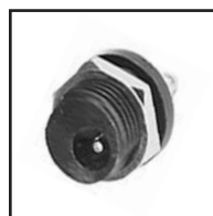
30-314 2.1mm I.D. X 5.5mm O.D. 30-315 2.5mm I.D. X 5.5mm O.D. Chassis mount coax power jack. Plastic housing. Mounts in 1/2" dia. hole. N/C switch.
