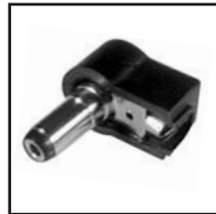
30-357 Right angle coax power plug. 2.5mm I.D., 5.5mm O.D. with solder terminals. .22" x .12" cable opening.
