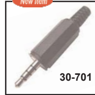
30-701 plastic 30-701A all metal 4 conductor 3.5mm Audio & Video Plug. Tip, ring 1, ring 2, sleeve, with strain relief. Cable opening .14"
