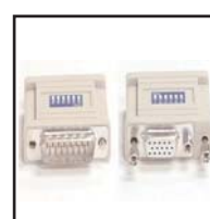
30-593 VGA to MAC adapter, 6 position Dip Switch For connecting Apple 15 pin (2 rows) to 15 pin (3 rows) D sub connectors. Supports Apple standard display modes including 13" color (640x480) 16" (832x- 624) 21" (1152x870). Dip switch selectable for different display modes.
