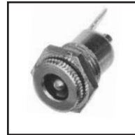
30-379 3.0mm I.D. 6.3mm O.D. chassis mount coax power jack. For 7/16" dia. hole in panels up to 3/16" thick.
