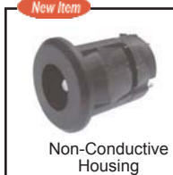
30-720-2.1 2.1mm version 30-720-2.5 2.5mm version Chassis mount snap-in coax power jack. Nickel plated connector with black molded trim. Isolated from ground, requires no hardware, solder style terminals. Mounts in .375" hole, up to .07" panel thickness
