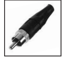
30-389 RCA Audio & Video male solderless connector with screw terminals, cable clamp and rubber boot. .24" cable opening.
