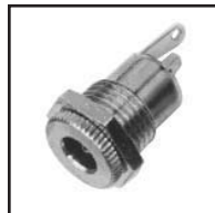
30-378 Japan 30-378-T Taiwan 2.5mm I.D. 5.5mm O.D. chassis mount coax power jack. For 7/16" dia. hole in panels up to 3/16" thick.
