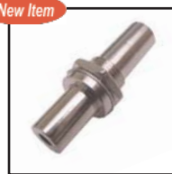
30-295 Nickel 30-295G Gold 3.5mm stereo female to female bulk head feed-thru Audio or infrared signal Jack. Mounts in 1/2" or 3/8" hole. Overall length 1.43". Available in gold or nickel 30-295-1/2 1/2" Nickel Version
