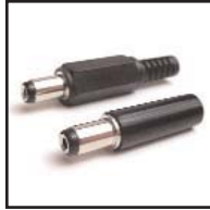
30-372 Coax power plug. 1.3mm I.D. 3.5mm O.D. 9.5mm long. .15" cable opening. 30-372-P With strain relief. .16" cable opening.
