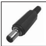
30-617-2.1 30-617-2.5 Locking DC power coax plug 5.5 O.D., 9.5mm long. Insert into 30-616 jack and twist clockwise to lock. Cable opening .14"
