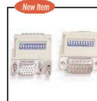
30-594 VGA to MAC adapter, 10 position Dip Switch For connecting Apple 15 pin D sub (2 rows) to 15 pin (3 rows) D sub connectors. Supports Apple standard display modes including 13" color (640x480) 16" (832x- 624) 21" (1152x870). Dip switch selectable for different display modes.
