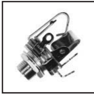
30-394 Stereo 1/4" Audio Jack. One Closed Circuit. .355" hole size.
