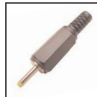
30-337 Coax AC/DC power plug 2.35mm O.D., .7mm I.D. .17" cable opening with strain relief.
