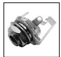
30-422 3.5 mm miniature closed circuit mono Audio Jack mounts in 1/4" hole, in panels up to 1/8" thick. Nickel plated. Bushing length .17".
