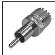
30-469 Coax universal jack adaptor. Adapts PL 259 to Motorola-type auto antenna plug or RCA-type phone plug.
