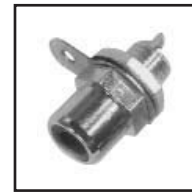
30-425-BK Black 30-425-RD Red RCA-type mini Audio Jack with hex nut grip, hex nut and solder lug. Single hole mount. 1/4" hole. 9mm hex base. Bushing length .27".
