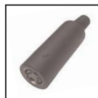
30-322J-4 (4 pin) 30-322J-6 (6 pin) 30-322J-8 (8 pin) Inline female mini din connector. Solder type inline female connector with strain relief. Shielded body with plastic cover.
