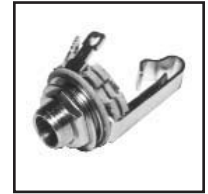
30-412 Closed Circuit 1/4" Mono Audio Jack. .35" x .29" bushing. .36" hole size, will work with standard .375" hole.
