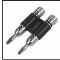
30-604-BK Black 30-604-RD Red Dual gold banana plugs. For up to 8 gauge wire. .15" cable opening. .075" centers.
