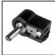
30-355 Right angle coax power plug. 1.3mm I.D., 3.5mm O.D. with solder terminals. .22" x .12" cable opening.
