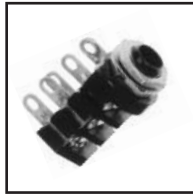
30-398 1/4" Audio Jack. 3-Circuit, 2 Closed. 3/8" bushing. Mounts in .355" hole.
