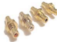
30-410-COLOR NICKEL 30-410G-COLOR GOLD Mounts in 1/2" hole. Bushing length .29" Overall length 1.3"
