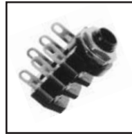
30-399 1/4" Audio Jack. 3-Circuit, 3 Closed. 3/8" bushing. Mounts in .355" hole.
