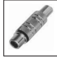
30-351 Red 30-353 White Gold plated RCA Audio & Video inline jack with color coded band, knurled barrel and strain relief .21" cable opening.
