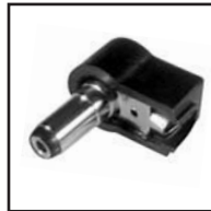
30-356 Right angle coax power plug. 2.1mm I.D., 5.5mm O.D. with solder terminals. .22" x .12" cable opening.
