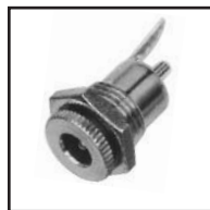
30-377 Japan 30-377-T Taiwan 2.1mm I.D. 5.5mm O.D. chassis mount coax power jack. Mounts 7/16" dia. hole in panels up to 3/16" thick.
