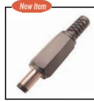
30-635 Coax AC/DC power plug 4.75mm O.D., 1.7mm I.D. .17" cable opening 30-632 same as 30-635 w/ O.D. of 4mm
