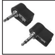
30-376-2.5 mono 30-386-2.5 stereo 2.5mm mono and stereo right angle mini Audio Plugs. Solder terminals with snap-on black PVC plastic body. .15" cable opening.
