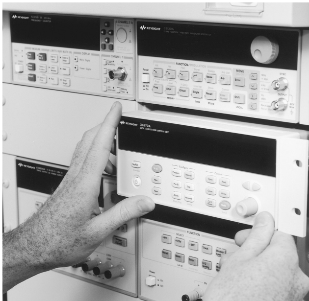
Low-cost switching system for automated testing
