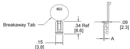
Note: #2216 B/A Scotchweld can be used to adhere keys.
