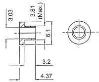
Dimensions : Millimetres Tolerance: 0.15mm
