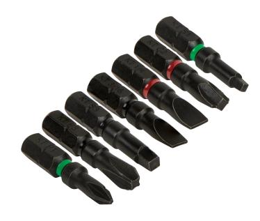
Klein Tools has designed a set of Impact Power Bits for the professional electrician. All the bits are made of high-impact rated S2 steel and color coded for easy identification. The 1-1/4-Inch (31.8 mm) long driver bits are easier to grip than a standard 1-Inch (25.4 mm) bit. You can find these bits along with additional size and tip bits in our Pro Impact Power Bit Set with Case (Cat. No. 32799).
