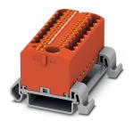
Distribution block, Block with horizontal alignment and integrated supply, the blocks can be bridged with one another via the conductor shaft, for corresponding plug-in bridges, see accessories, nom. voltage: 690 V, nominal current: 24 A, connection method: Push-in connection, Push-in connection, number of connections: 19, cross section: 0.14 mm² - 4 mm², AWG: 26 - 12, width: 56.5 mm, color: red, mounting type: NS 35/7,5, NS 35/15
