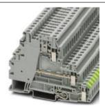
Ground modular terminal block, nom. voltage: 500 V, nominal current: 28 A, connection method: Screw connection, cross section:  $0.14 \text{ mm}^2$  -  $6 \text{ mm}^2$ , AWG: 26 - 10, length: 92.7 mm, width: 6.2 mm, color: gray, mounting: NS 35/7.5, NS 35/15, nom. voltage: 500 V
