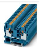
Feed-through terminal block, nom. voltage: 1000 V, nominal current: 57 A, connection method: Push-in connection, Rated cross section: 10 mm², cross section: 0.5 mm² - 16 mm², mounting type: NS 35/7,5, NS 35/15, color: blue
