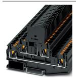
Fuse modular terminal block, fuse type: Glass / ceramics / ..., connection method: Push-in connection, cross section:  $0.2 \text{ mm}^2$ -  $6 \text{ mm}^2$ , AWG: 24 - 10, nominal current: 28 A, nom. voltage: 500 V, width: 6.2 mm, fuse type: G /  $5 \times 20$ , mounting type: NS 35/7.5, NS 35/1.5, color: black
