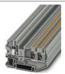
Feed-through terminal block, connection method: Push-in connection, Screw connection, cross section: 0.2 mm<sup>2</sup> - 6 mm<sup>2</sup>, AWG: 24 - 12, width: 6.2 mm, color: gray, mounting: NS 35/7,5, NS 35/15
