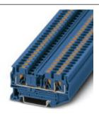
Feed-through terminal block, Connection method: Push-in connection, Cross section: 0.2 mm<sup>2</sup> - 6 mm<sup>2</sup>, AWG: 24 - 10, Width: 6.2 mm, Color: blue, Mounting type: NS 35/7,5, NS 35/15
