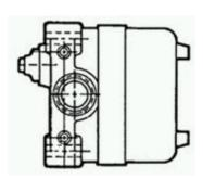
**Explosion-Proof Limit Switches Series CX: Short Housing: Top Plunger; 1NC 1NO SPDT Snap Action; Number of** internal basic switches BZ: 1; 0.75 in -14NPT conduit
