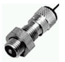
High Temperature VRS Sensor, 6,4 mm [0.250 in] M8 diameter, 4.7 Vp -p, -40 °C to 230 °C [-40 °F to 450 °F], 36 DP (module 0.70) or coarser, 70 kHz, 23 mm [0.90 in] approx. length
