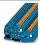
Feed-through terminal block, Connection type: Quick connection, Spring-cage connection, Cross section: 0.25 mm² - 1.5 mm², AWG :24- 16, Width: 5.2 mm, Color: blue, Mounting: NS 35/7,5, NS 35/15
