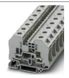
Bolt connection terminal block, Connection type: Bolt connection, Cross section: 0.1 mm<sup>2</sup> - 6 mm<sup>2</sup>, AWG: 26 - 10, Nominal current: 41 A, Nominal voltage: 1000 V, Length: 66 mm, Width: 16.3 mm, Color: gray, Assembly: NS 35/7,5, NS 35/15
