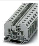
Bolt connection terminal block, Connection type: Bolt connection, Cross section: 0.1 mm² - 2.5 mm², AWG: 26 - 14, Nominal current: 24 A, Nominal voltage: 1000 V, Length: 66 mm, Width: 12.3 mm, Color: gray, Assembly: NS 35/7,5, NS 35/15
