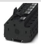
Fuse modular terminal block, Connection method: Screw connection, Cross section: 1.5 mm<sup>2</sup>- 25 mm<sup>2</sup>, AWG: 16 - 4, Nominal current: 32 A, Nominal voltage: 690 V, Width: 36 mm, Fuse type: Class CC, Fuse type: Glass, Mounting type: NS 35/7,5, NS 35/15, Color: black
